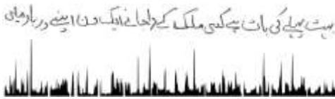
Figure 1-9 Projection profile of printed Urdu text
